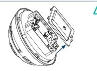
Remove the battery compartment cover on the base on the detector
